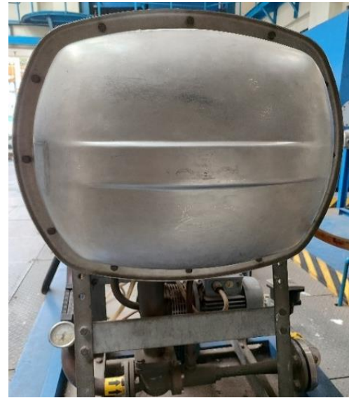
Gambar 3. Fresh Water Generator
