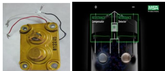
Gambar 1. Gas detector catalytic combustion [2][3]
