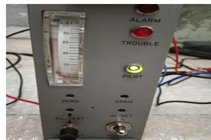
Gambar 4. Module gas detector merk komyo, type FMA-IG 14 W [1]
