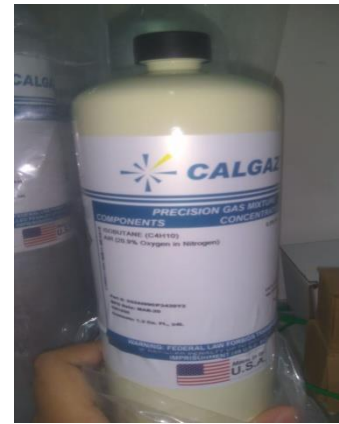
Gambar 9. Tabung gas Calgaz part# :X02A199CP3439Y2 Component isobutane (C4H10), air (20,9 % oxygen in nitrogen) [3].
